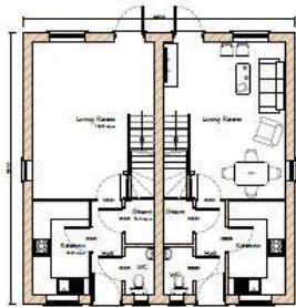
PROPOSED GROUND FLOOR PLAN - PLOTS 6/7 SCALE 1:100
